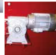
MTX_A agitator device for homogenizing straw mixed with molasses, removes the lumps.
