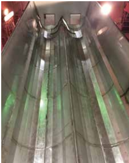
AISI 316 L, covered and closed insulated MTX_ETH: Hydrator for chemical processes used for Bio Ethanol production from straw. This is also used on buffer mixers for biogas production.
