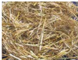
Straw after our RBS straw shredder system, shortening the straw down to 100 mm.
