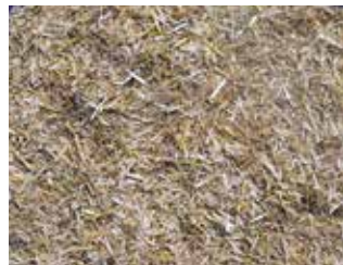
Straw after being processed in a straw mill with 10 mm screen.
