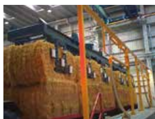
Load weighing and moist control
