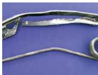
Handling of larger steel contaminations is possible without any major breakdown on the line.
