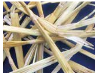
Only a straw mill can crush the nodes in the straw and open up the straw tube, thus making the straw more moist absorbent and giving access for further processing.
