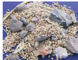
Above picture shows the normal contamination's found in our pneumatic stone trap.
